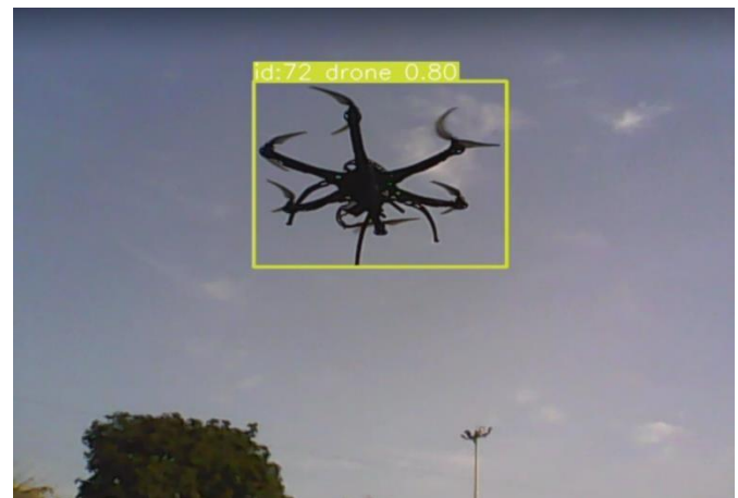
Figure 4: Real-time drone detection using YOLOv8
