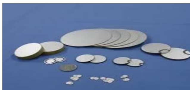
Fig. 2 Piezoelectric Crystal Discs. Note that “Fig.” shows Piezoelectric Crystal Discs which is a thin, circular piece of piezoelectric material, typically made from quartz, lead zirconate titanate (PZT), or other piezoelectric ceramics [10].
