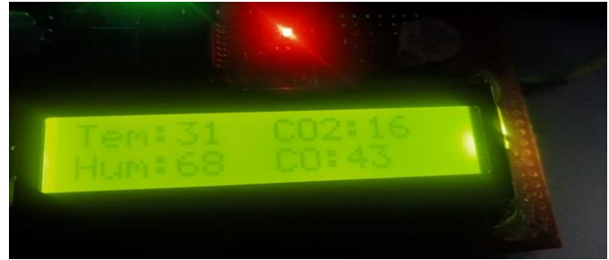
Fig 4: Temperature, Humidity, CO 2 , CO values
